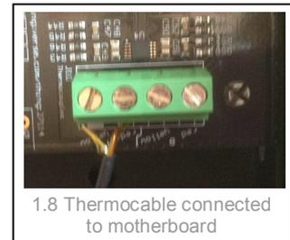
1.8 Thermocable connected to motherboard
