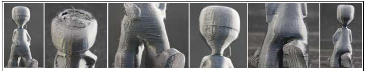
1.3 Print quality impaired without filament fan. Notice the slight droop on the foot, chin, thigh and stomach, and the hole in the head!
