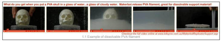
"We've come up with a few uses for water soluble components here at the BotCave, and the possibilities are amazing! Some of the applications include: making soluble molds, building removable support structures, biotechnology applications, or fascinating science experiments of your own creation. It is pretty awesome for video and visual effects projects as well.
